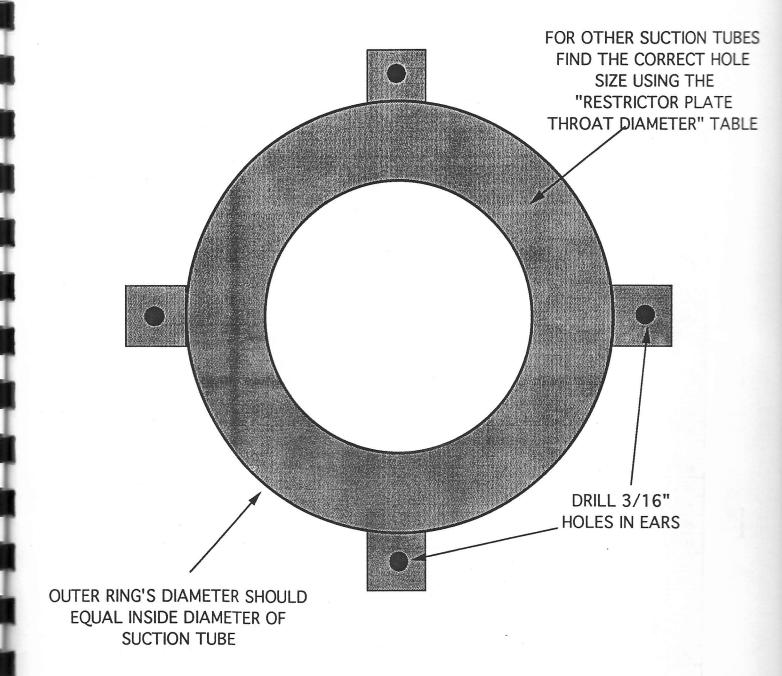
300 CFM RESTRICTOR PLATE TEMPLATE FOR THE WEEDEATER® SUCTION TUBE
